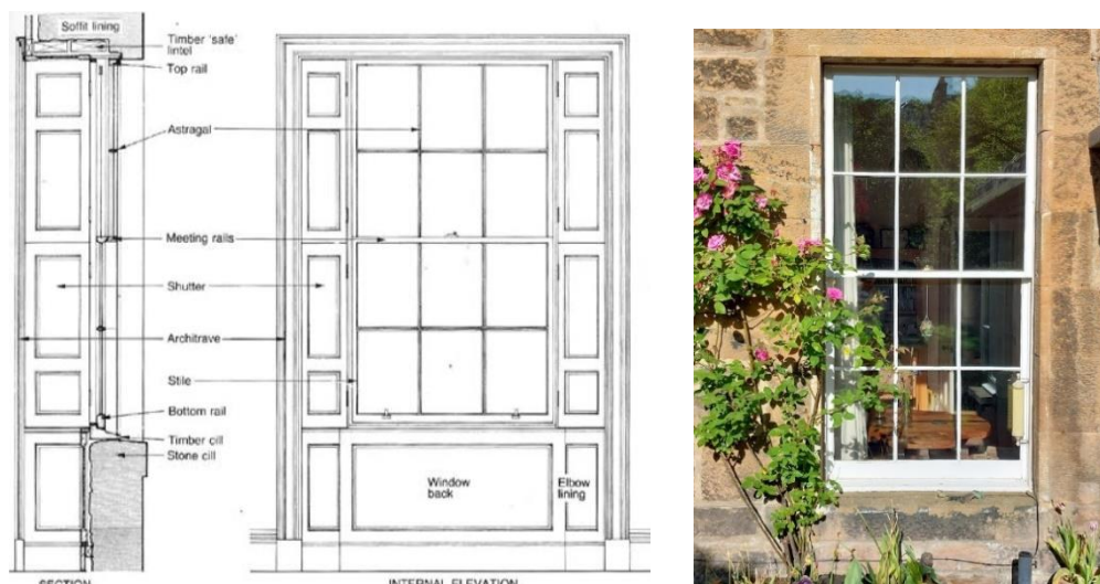
Figure 1: Details of window structure and external view of window with thin double glazing installed
